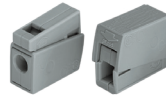
224-101 / 2-con Installation side:- 1 - 2.5mm 2 "s" Lighting side:- 0.5 - 2.5mm 2 "s" / "f-st" 400V/4kV/2' - 24A
