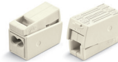
224-112 / 3-con Installation side:- 1 - 2.5mm 2 "s" Lighting side:- 0.5 - 2.5mm 2 "s" / "f-st" 400V/4kV/2' - 24A
