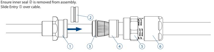
**NOTE:** A spare entry component could be used to clamp the armourings, which removes the need to remove the inner seal of the gland to be assembled.
