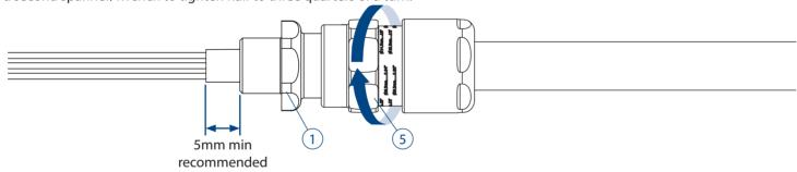
**NOTE:** Support the cable to prevent it twisting. To aid wiring inside the enclosure, it may be beneficial to strip the inner sheath as shown above.
